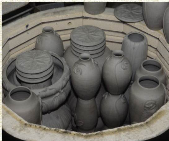
A kiln loaded with green ware
